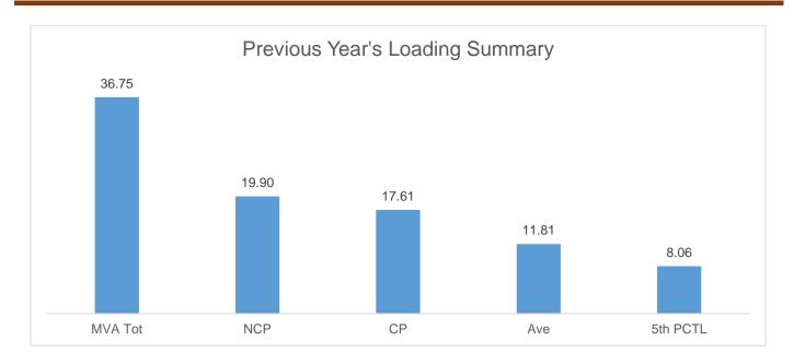
The Non-coincident Peak Demand is <u>19.90</u> MW, which is around <u>54.16</u>% of the total substation capacity of <u>36.75</u> MVA at a power factor of <u>99%</u>. The load factor or the ratio between the Average Load of <u>11.81</u> MW and the Non-coincident Peak Demand is <u>59.5</u>% of. A safe estimate of the true minimum load is the fifth percentile load of <u>8.06</u> MW which is <u>40.5</u>% of the Non-coincident Peak Demand.
